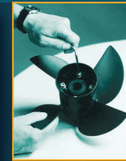
3. Tighten bolts w/ allen wrench.
