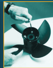
4. Tighten bolts w/ allen wrench.
