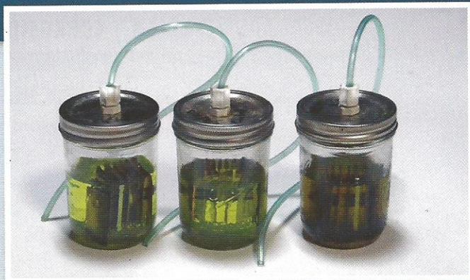
Our lab testing was modeled after an automotive industry test for evaluating the performance of engine coolants.
